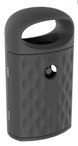
Litter bin made of 4mm-thickness high density polyethylene, resistant to UV rays, chemical agents and impacts. Inner polyethylene bucket with 80L capacity and separated stainless steel ashtray (the fag-ends are not thrown in the same container). Stainless steel screws, AISI 304. Finishing: Wrinkled finishing (stickers cannot properly be glued). Black forge colour. Recommended anchoring: Four Ø10 expansion bolts, depending on the surface.
