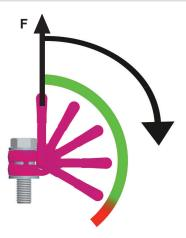
Pic. 6: Pivoting in load direction
