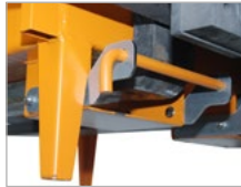
Secured by bolt to prevent slipping from the forklift truck
