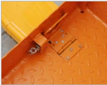
Safety mechanism for a straddle stacker
