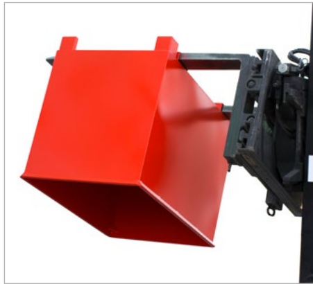
Emptying using a forklift rotator
