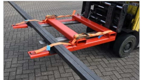
Position: load at the front for loading and unloading
