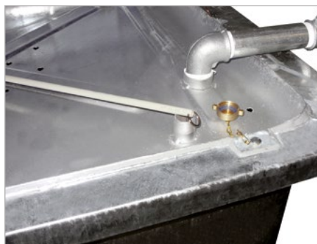
Dipstick to control the fill level
