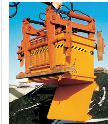
BC with brick clamp operated trap door
