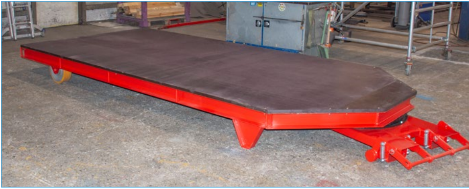
STS with anti-slip "Betosieb" boards
