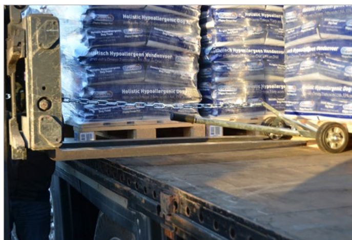
Drawing the pallet into the "front row" using a forklift truck
